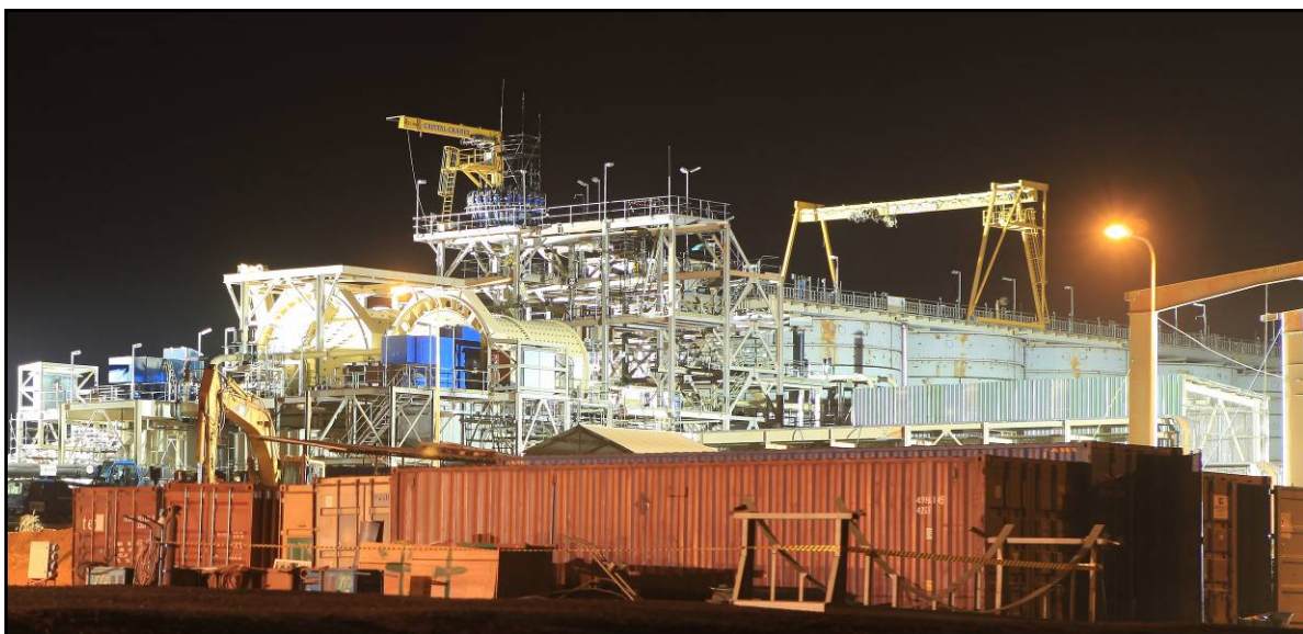
Plant showing SAG and ball mills in yellow and CIL tanks in background
