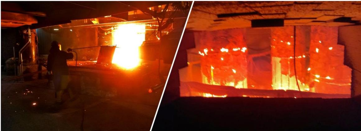
*Slag tapping underway at the TiZir Titanium & Iron ilmenite upgrading facility, Tyssedal, Norway*
